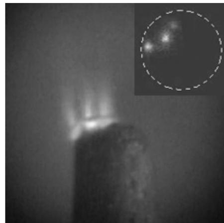
Fig. 3. Side photograph of the cathode during discharge.
