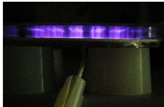
Fig. 7. Time-averaged photograph of the DBD coupled with surface discharge
