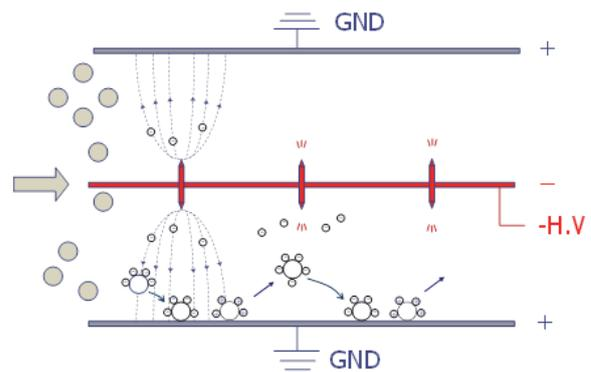
Fig. 2. Concept for low resistive particle reentrainment.
