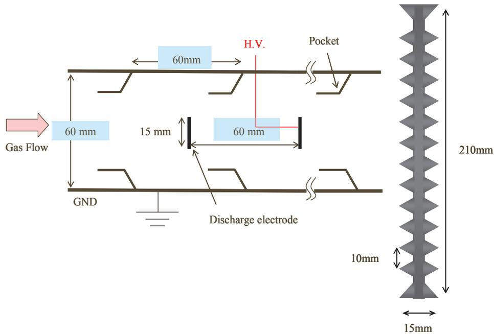
Fig. 1. EHD assisted ESP configuration.
